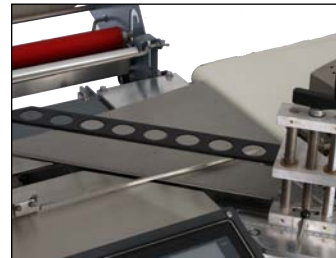
Adjustable Inverting Head (HS-1 and HS-3 only)
